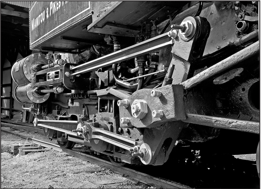
A view of the unorthodox Vaclain valve gear and rods on Manitou & Pikes Peak Railway No. 4. – Photo © 2010 Joe McMillan
